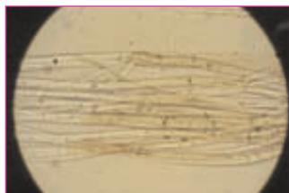
Figure 9. Example of how the color ends abruptly with an increase in optical density on some fibrils. One vertical end just above the main smudge at the center is heavily coated and colored.
