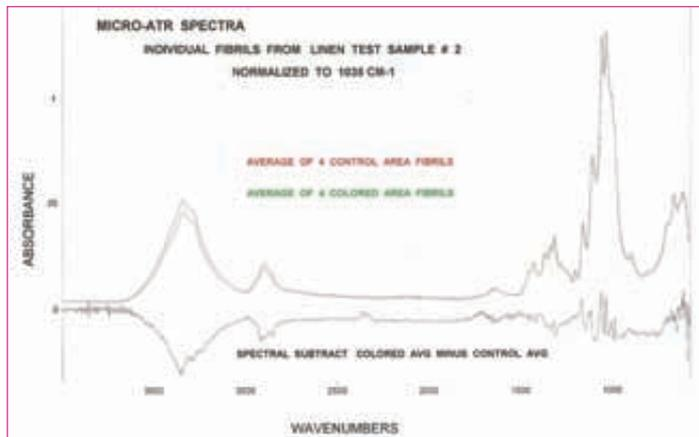
Figure 5. Micro-ATR-FTIR of sub-sample indicated dehydration in discolored regions similar to Shroud image fibers.
